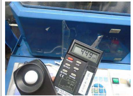
Photo 22) NC4.7.1 Lighting result on knitting machine
